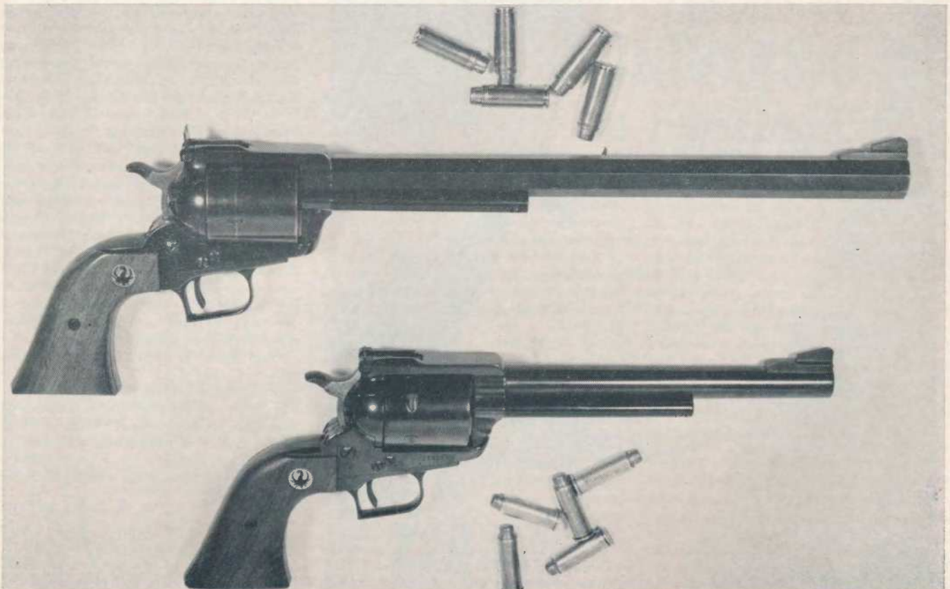
Dick Casull's conversion of a Ruger Super Blackhawk (top), with a standard .44 Magnum Ruger. The ejector rod housing is soldered to flat of barrel. Heavy recoil hasn't shaken one loose yet.
