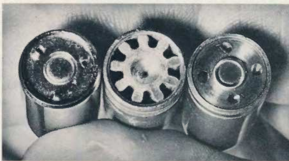
Left: Shown here are three of the jet nozzle variations used in test. Right: Bob Mainhardt displays one of his miniature Lancejet rockets.
