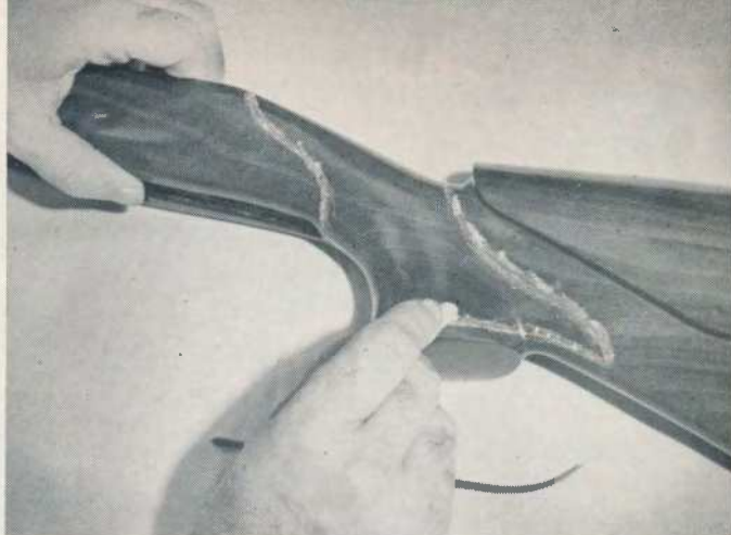
To compliment a particular gun, the checkering pattern should be sketched on the stock itself.
