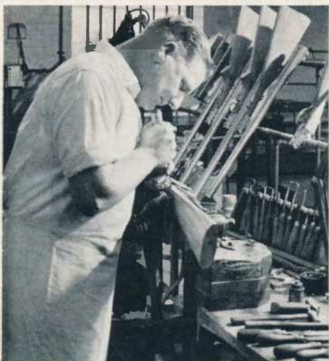
Many hours of hand labor go into each Webley shotgun, fitting various parts together precisely.
