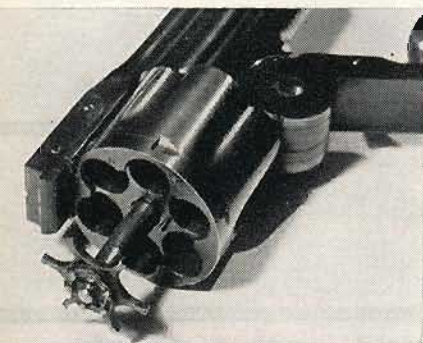
Ratchet star fit in mortise affects cylinder side-rock.
