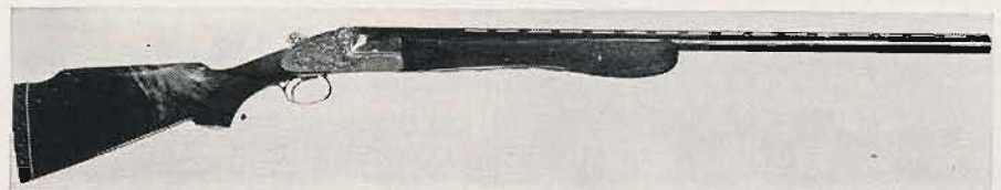
Typical trap single gun shows straight stock lines and long elevated rib to reduce heat-haze on viewing flying targets. Stock comb raises head height.
