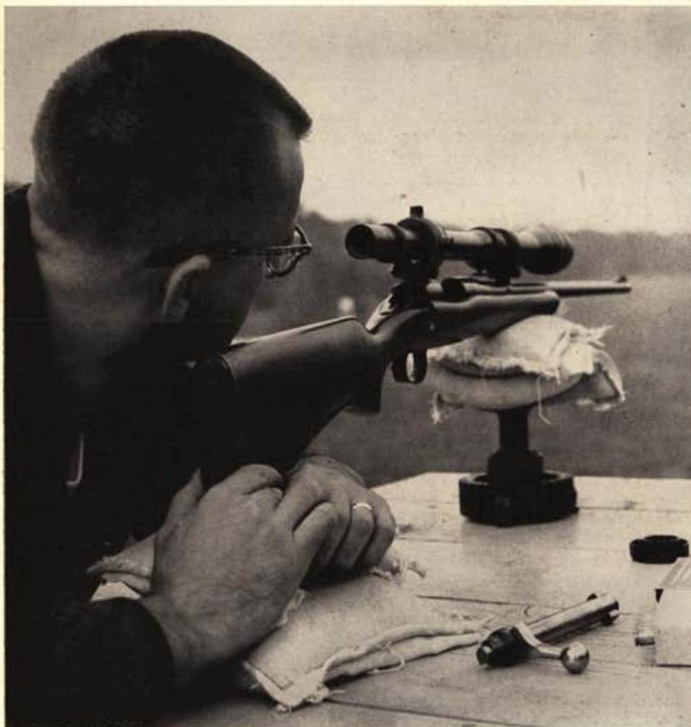
Using improvised bench rest and with bolt out for bore-sighting, author gets light bolt action ready for tests.
