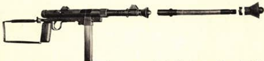
New model of Carl Gustave burp gun made in Sweden and imported by Interarmco has special barrel with plastic bullets to give realistic safe practice.
