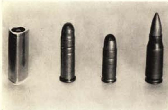
Dardick tround is equivalent to .38 Spl., may adapt 9 mm ammo to gun. At right, short German 7.9 was also made of combustible propellant in WW II.
