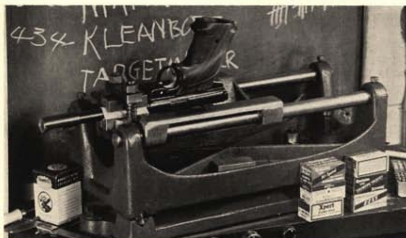
Carbide lamp is used for smoking sights to make them stand out on target paper. Smoke does not hurt finish of gun or Lee muzzle brake on .45 automatic. Bottom, Ruger .22 is tested for choice of ammo in Potter machine rest.
