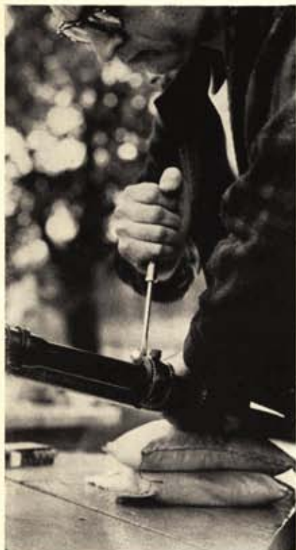
Mounts had to be seated extra tight to buck inertia of the heavy scope.
