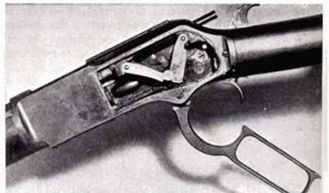
Middle joint of Winchester 76's toggle lock is collapsed by moving finger lever forward, draws bolt back.
