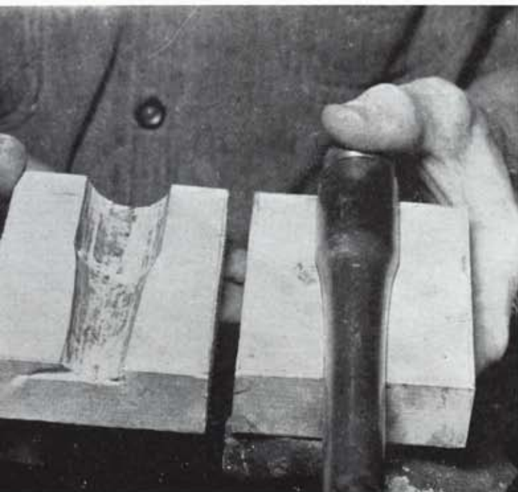
Barrel must be gripped solidly and without slipping in hardwood vise jaws which have been inletted to fit it.
