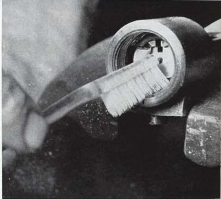
Barrel and receiver threads must be clean. Toothbrush and "carbona" will dissolve grease and remove grit.
