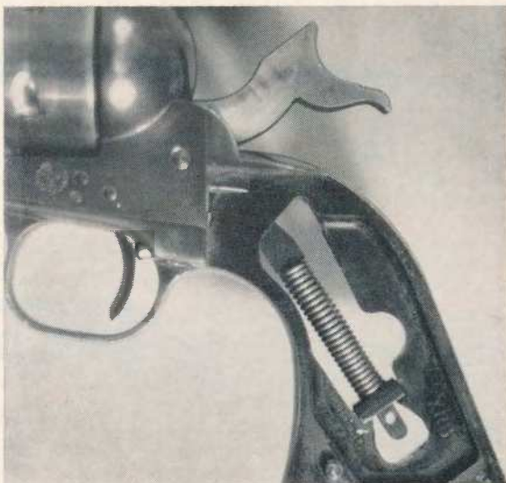
Ruger's SA mainspring is removed by cocking hammer and inserting pin in a hole in guide.
