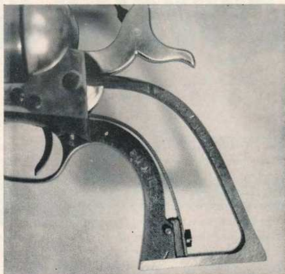
A thick leather pad under the mainspring on a Colt SA dampens whip, lightens cocking action.
