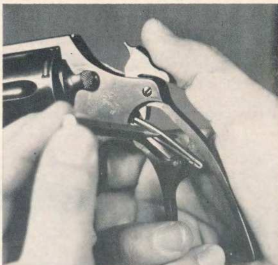
DA Colt action can be lightened by cocking the hammer with a small rod inside the mainspring.
