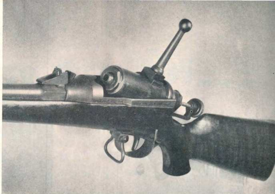
The bolt tips rearward to facilitate loading.
