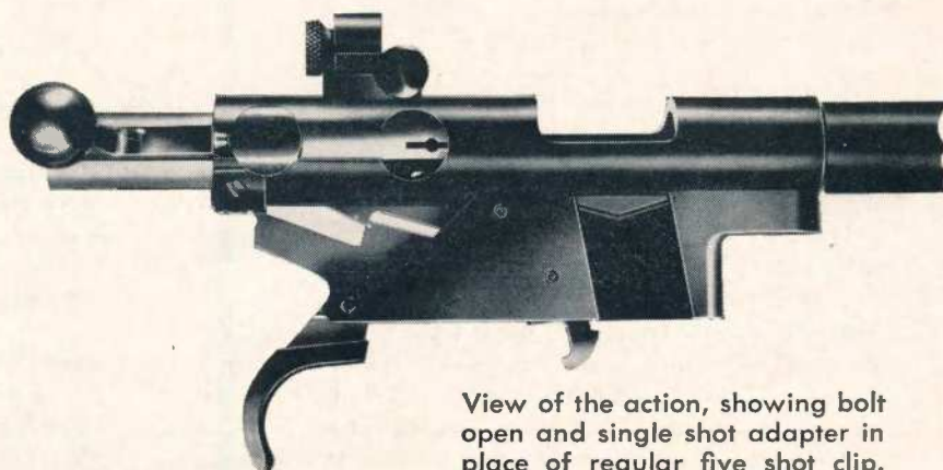
Inner portion of safety prevents the bolt from moving back and, at same time, locks trigger.
