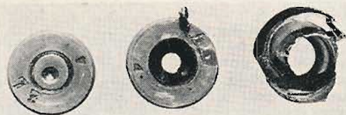
Normal load; hot load which blew primer; excessive charge blew case, wrecked rifle.
