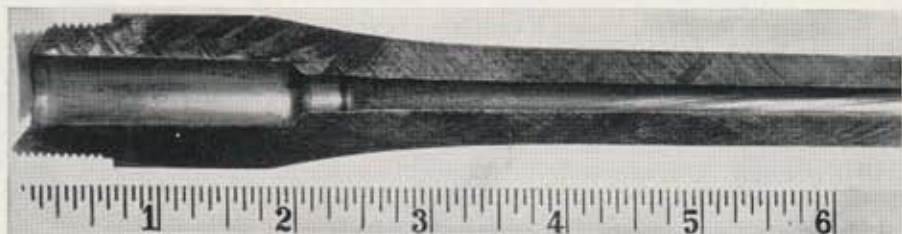
Condor bore after 1025 shots is eroded at case throat; heat-checked for 2".
