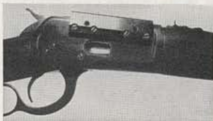
Scope mount best for levers like '94 is Weaver's side type, (shown on M92).
