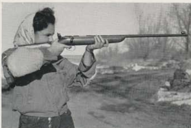
Short 11½" stock is just right for 14-year old girl, if drop is right, but barrel shown is too long for steady hold.
