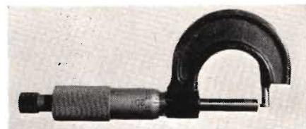
Micrometer with nail head silvered on makes good neck thickness gauge.
