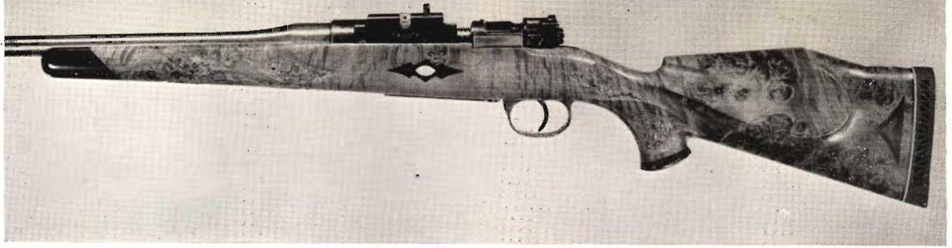
Before and after of a stock blank. Rare maple burl blank (right) was seasoned 25 years, shaped into combination of man made and natural art as stock for 7mm by N. H. Hultgren.
