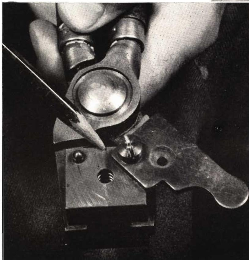
Inspect mould for warpage. Parting line should be mere crack in good mould, like Ideal single cavity type used in story.
