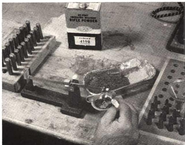
Weighing layout (hold to .01 grain) has capped hulls end up at left, powder scale and fixin's, charged cases right.
