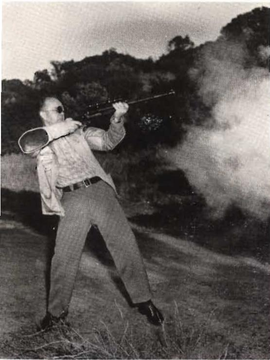
Kick of 8-bore rifle, 1700 grain bullet and 165 lbs. recoil proves Buehler scope mount can take it.
