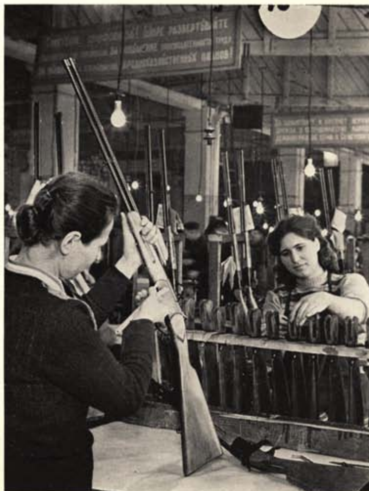
Inspector checks breech fit on new model Byelka combination gun made in Izhevsk plant. Top bore is 32 gauge, bottom is rifled smallbore. Weapon breaks by pushing guard bow, is liked in Siberia.
