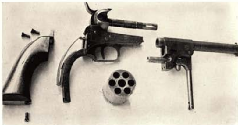
Sample found in Austria has V spring like Dragoon but improved grip strap design.
