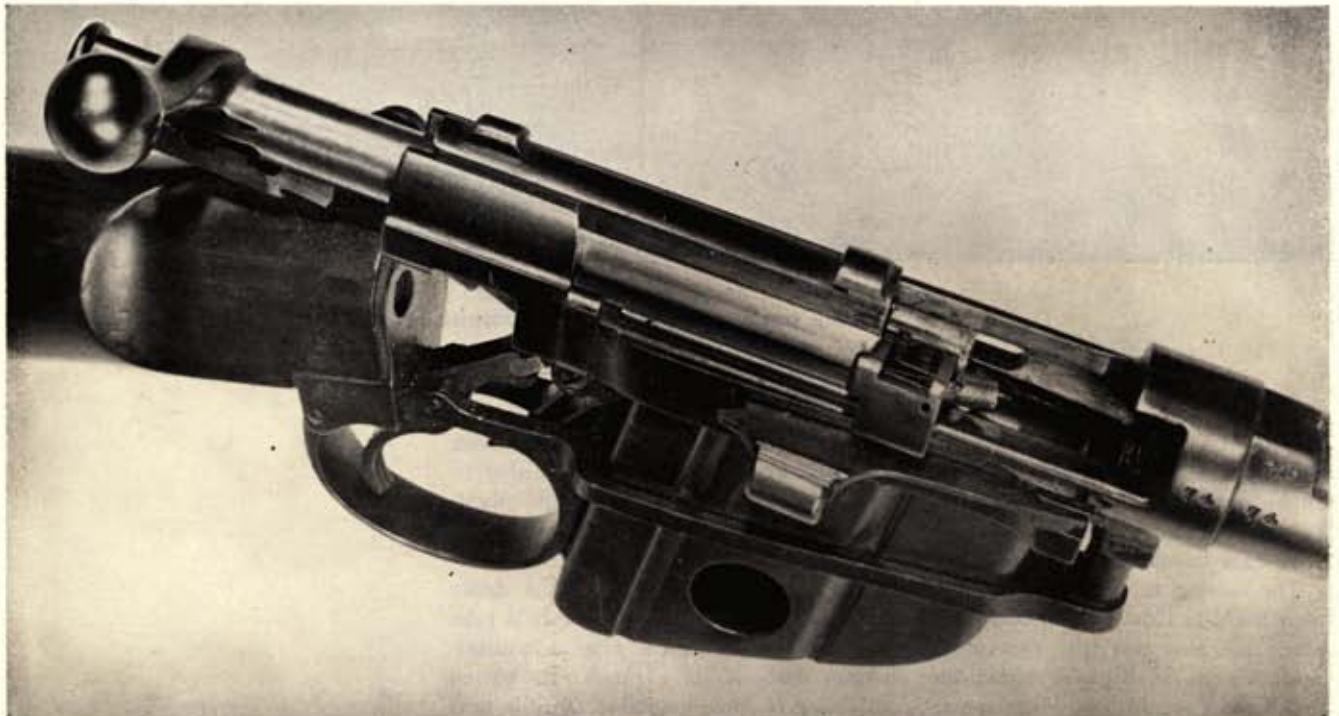
Cutaway armorer's model of Lee action shows trigger simplicity, bolt handle at rear for fast shooting, which endeared it to British military authorities.
