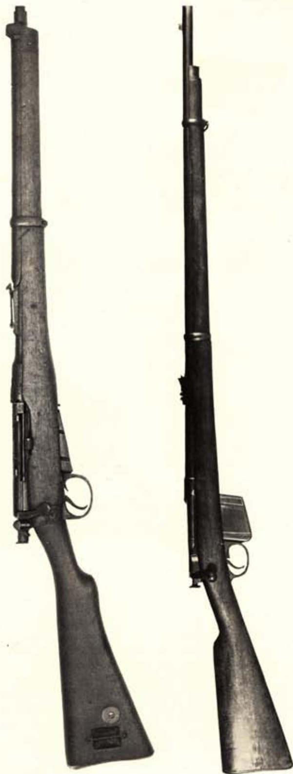
Many varieties of basic Lee bolt action were produced, such as this flat-handled cavalry .303 British carbine in Martin Retting collection. At right is first Lee rifle, experimental .43 military musket made at Sharps Rifle Co. in Bridgeport before Sharps firm folded in 1880's.
