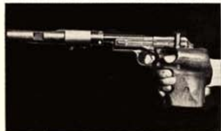
Margolin pistol with hand-in-cast grips and muzzle brake, helped Red shooters win many international matches.
