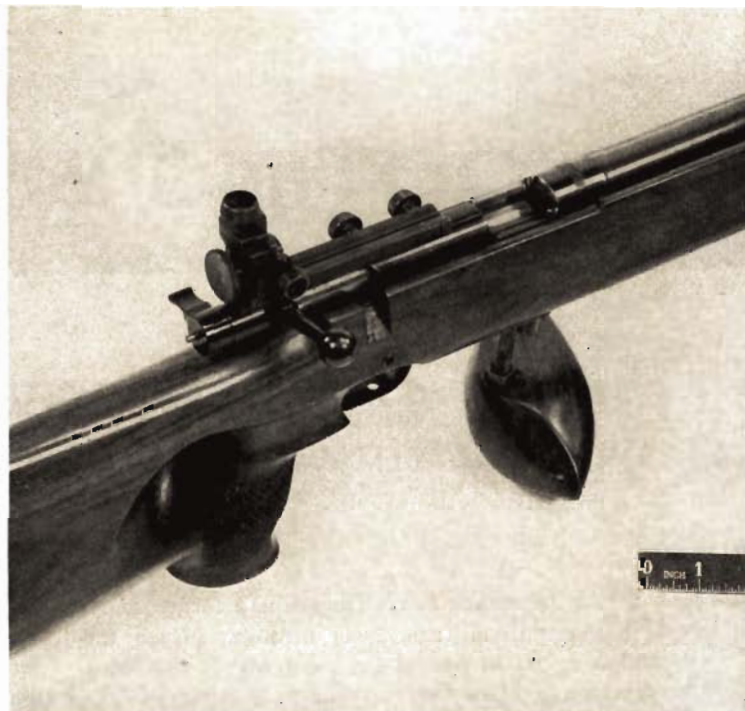
Anschutz free rifle receiver is round like smallbore Mausers. Trigger adjusting screw hole is by bolt cut.
