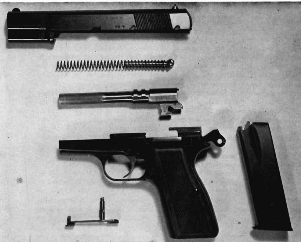
Easily-stripped Hi-Power shows changes from earlier models in design of fixed cam lug on barrel and fixed bushing in slide. Recoil spring has guide which holds take-down lever in place. Fat clip holds 13 shots, most of any pistol.
