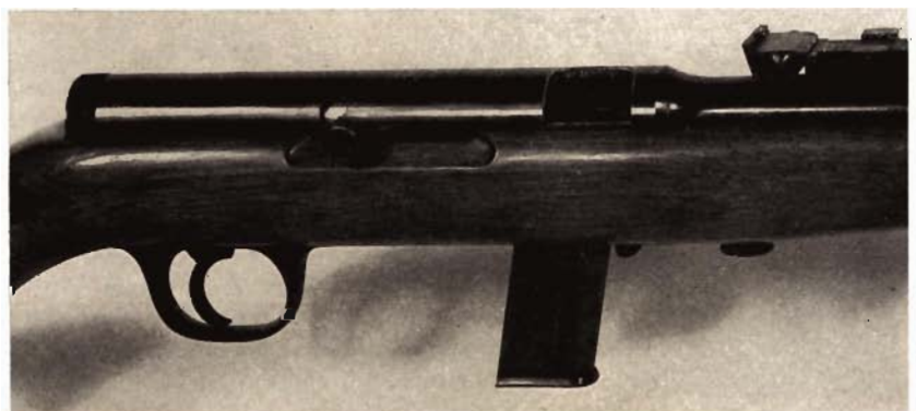
Gevarm .22 in cocked position has bolt open, feeds from clip on closing.
