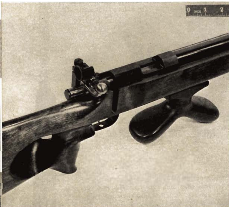
Finnish Lion smallbore rifle has bolt handle which locks down into rear of receiver machined from solid steel.
