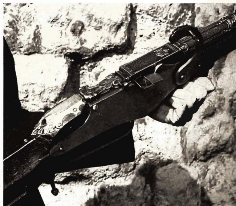
Breech-loading gun made for Henry VIII is shown at left with action open and at right with action closed ready for firing. Lock is not one with which gun was originally fitted, is a match-lock added early in 19th century replacing wheel lock.
