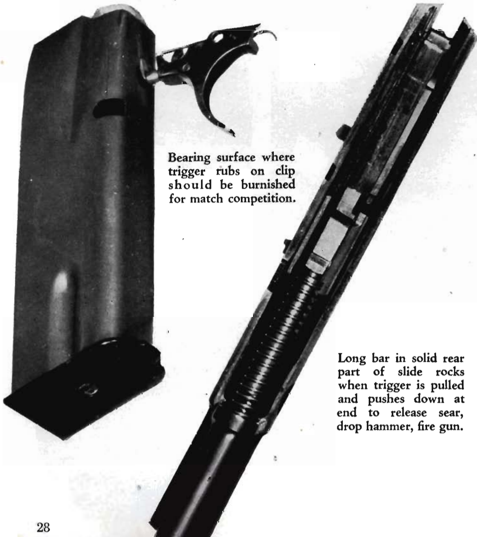
Easily-stripped Hi-Power shows changes from earlier models in design of fixed cam lug on barrel and fixed bushing in slide. Recoil spring has guide which holds take-down lever in place. Fat clip holds 13 shots, most of any pistol.
