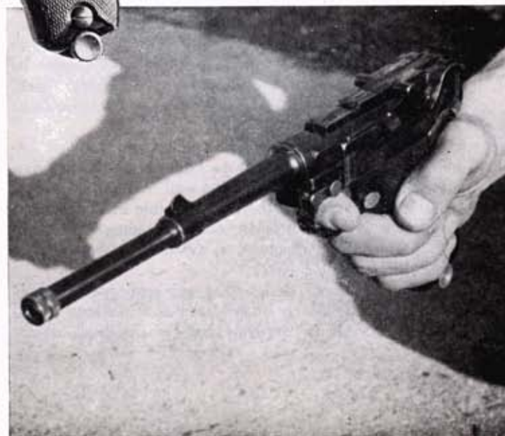
Erma sub-caliber unit changes Luger to .22 by placing new unit in barrel.
