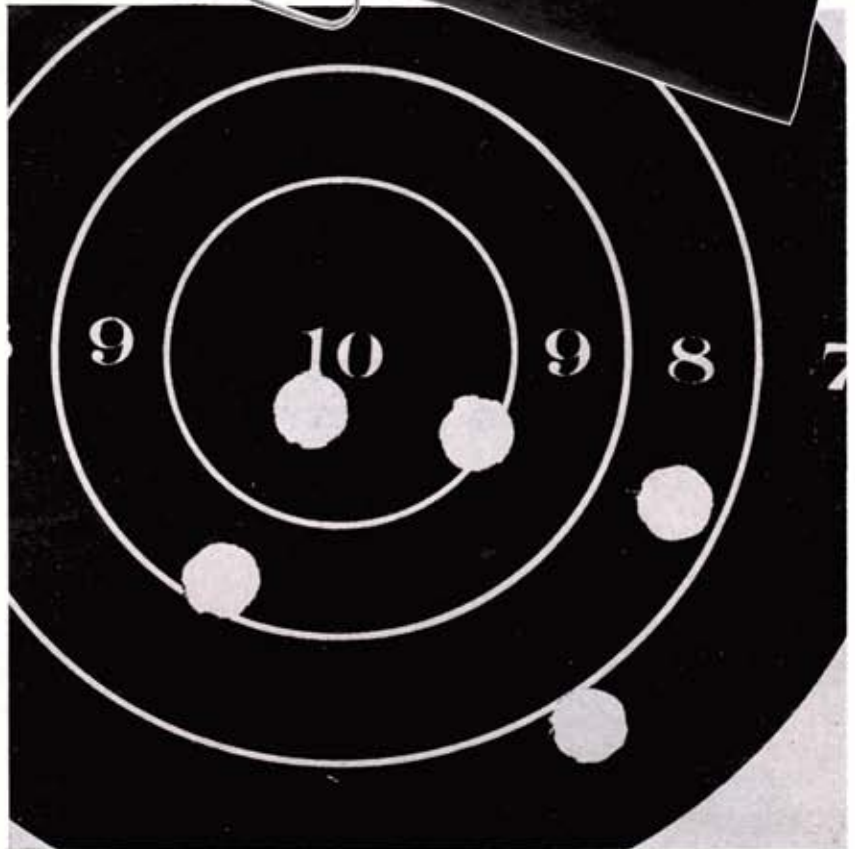
A 2\frac{3}{8} " group at 100 yards by Winchester Model 92 that has been chambered for .357 Magnum cartridge is as good as most sporting rifles.
