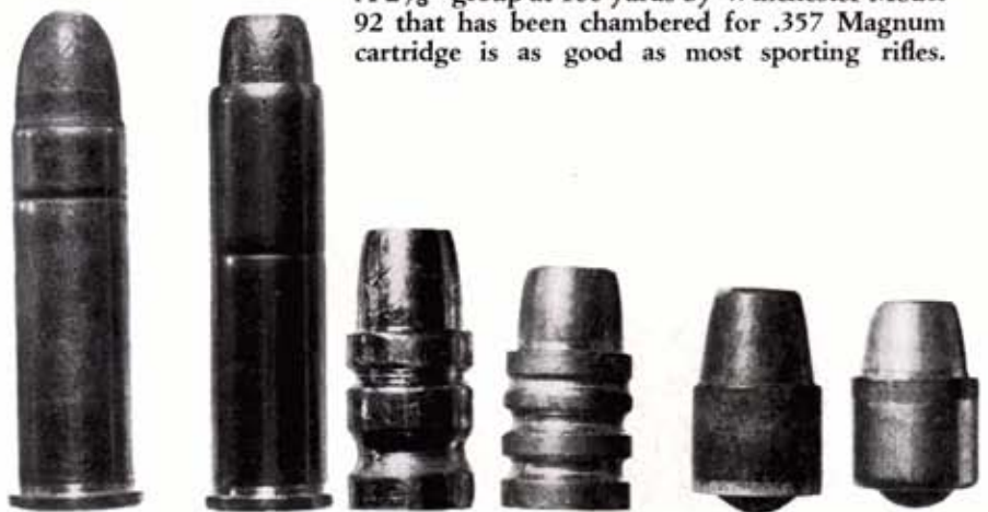
Standard .38s and .357s will feed okay when guides are altered. Test bullets (L to R) are Keith, Lyman standard Magnum, Protobore with zinc base, and the new Harvey Jugular Express. Bullet tips show cross cuts from sizing punch on noses of Keith, Sharpe, Harvey, and Bellah's extra large hollowpoint.
