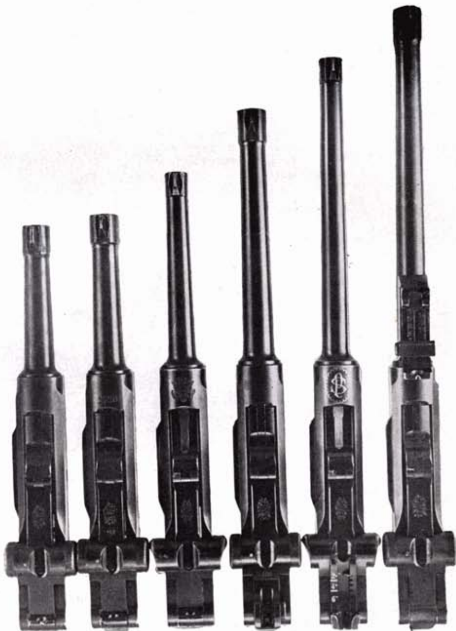
Luger barrels and types are (left to right) post-WWI .30 commercial, 9mm dated military, .30 M1900 commercial, Navy 6" model 1904, target model with special .30 barrel, and regular M1917 for stock with 8" 9mm barrel.
