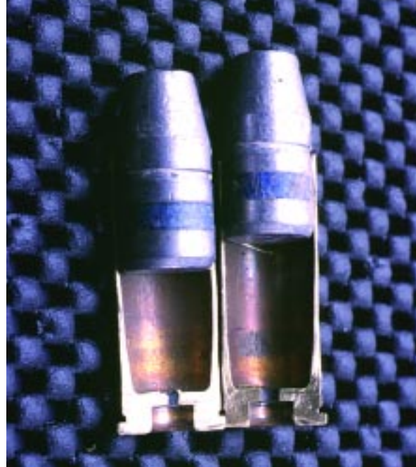
36 Seating your bullets out close to the rifling can improve accuracy, but seating too deep can be an invitation to disaster.
