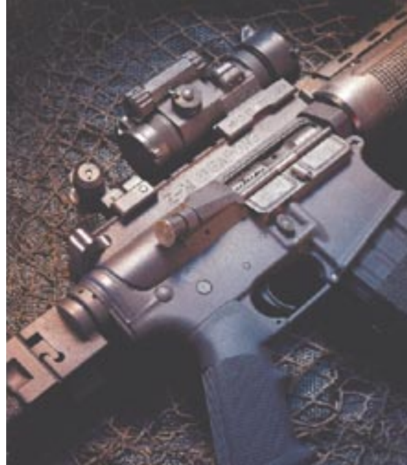
40 The recoil mechanism employed by ZM Weapons allows the LR-300 to carry a true folding stock, making it the most compact AR available.
